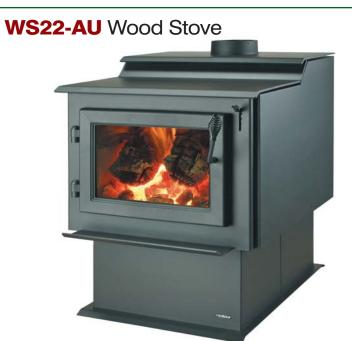
The WS22 features 6mm steel construction, a wide opening, an air wash system to keep the glass clean and a secondary wood combustion system to give you cleaner burns and less maintenance.
