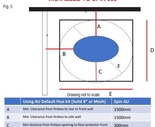
NOTE: HEAT SHIELD REQUIREMENTS FOR HEAT SENSITIVE WALLS
