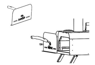
4. Attach handle to pellet burn basket with 2 x bolt and 2 x nut. Nut goes to inside of basket.
