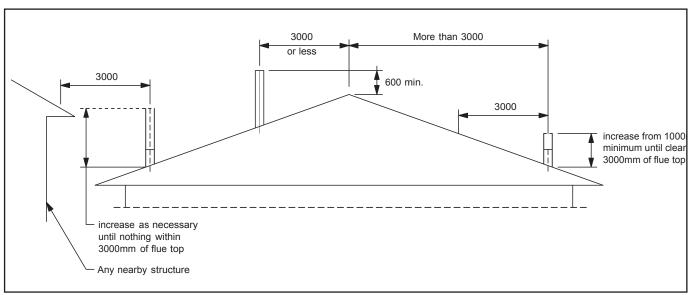
Figure 16.1 Minimum Height of Flue System Exit
