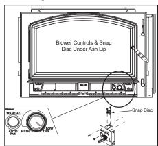
Figure 7.1 Snap Disc Location
