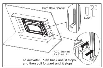
Figure 5.1 Start-up and Burn Rate Air Controls
