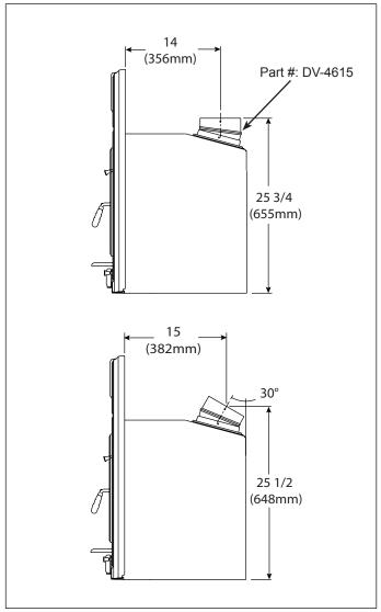
Figure 12.3 - Side View With Optional Flue Adapter
