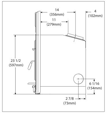
Figure 12.4 - Side View Without Optional Flue Adapter
